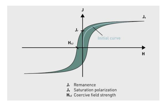
For magnetization into saturation polarization Js, a magnetization field of up to 200 kA/m is available. Additionally a pulse magnetization of 450 kA/m for hard magnetic specimen with  $H_{cJ}$  more than 50 kA/m is available as an option.
