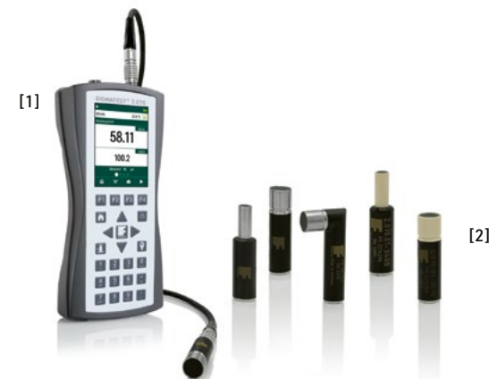
[1] SIGMATEST 2.070 [2] Conductivity probes
